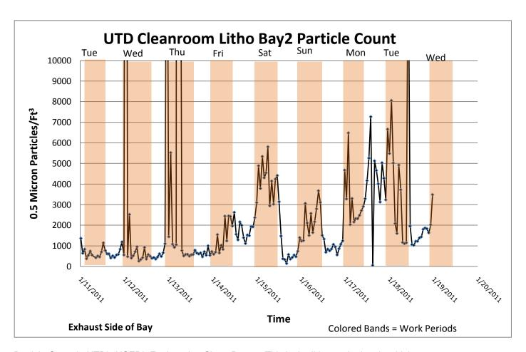
Particle Count in UTD's NSERL Engineering Clean Room. This is the lithography bay in which there is rather intense people activity, thus the particle count is high during working hours (color bands). Note that the Class 10,000 particles per cubic foot designation is based on 0.5 micron sized particles
